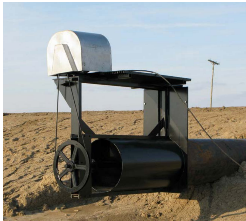
Figure 2 (left). Waterwheel design tested on commercial catfish ponds. Figure 3 (right). Screw-pump design tested on commercial catfish ponds.
