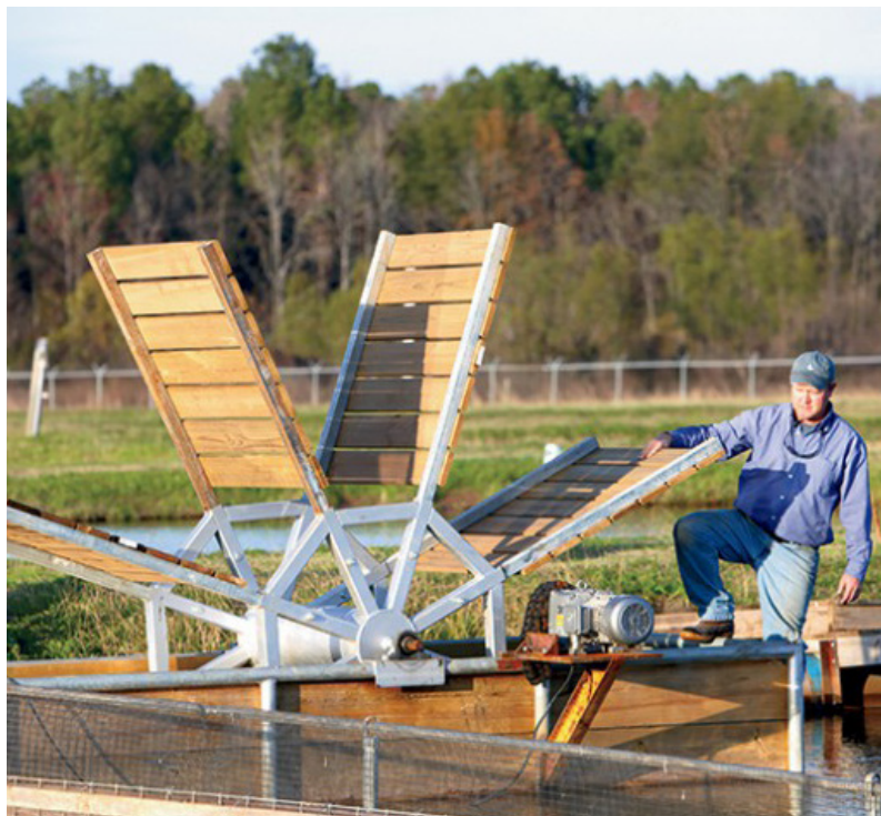
Figure 2 (left). Waterwheel design tested on commercial catfish ponds. Figure 3 (right). Screw-pump design tested on commercial catfish ponds.
